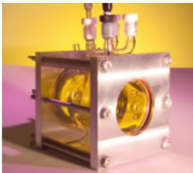
Photoreactor for high temperature solar powered hydrogen production.
