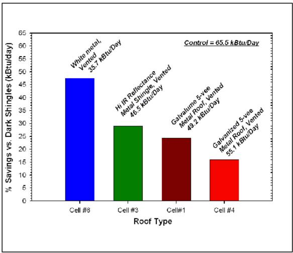
Figure 10. Percentage savings in daily total roof/attic related heat gain.
