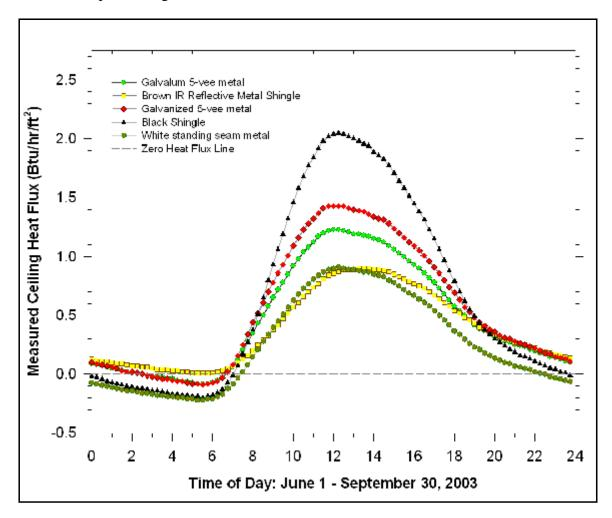
Figure 6. Measured average ceiling heat flux over the summer of 2003.
