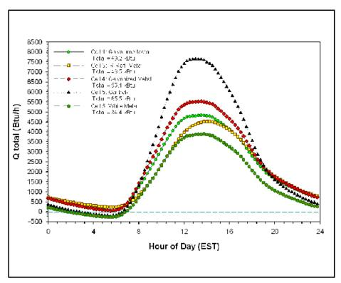
**Figure E-2.** Estimated combined impact of duct heat gain, air leakage from the attic to conditioned space and ceiling heat flux on space cooling needs on an average summer day in a 2,000 ft<sup>2</sup> home.
