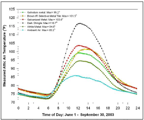
Figure 5. Measured average mid-attic air temperatures over the 2003 summer period.
