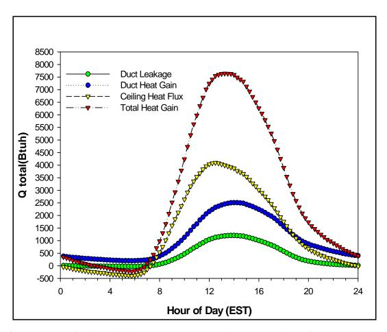
**Figure 9.** Components of estimated daily heat gain due to the duct heat gain, air leakage from the attic to the conditioned space and ceiling heat flux for Cell #5.
