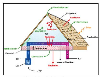
Figure 1. Vented attic thermal processes
