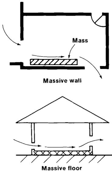
Locate openings close to massive wall or floor.
