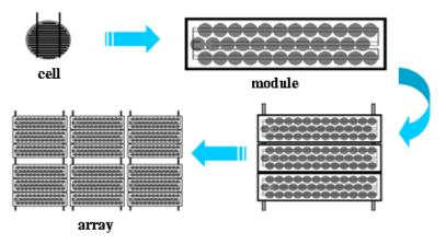
**Photovoltaic array** - The array which is made up of several photovoltaic modules converts or transforms sunlight directly into electric current. Like batteries, the current they produce is direct current (DC).
