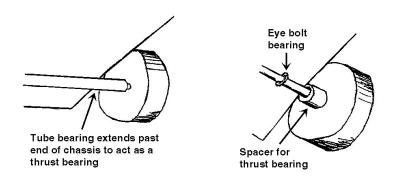
12. If there is something around the axles that let the center portion of the wheel touch first, the drag will be lower than if the outer part of the wheel touches. To demonstrate this,
