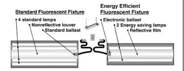
New fluorescent fixtures with energy-saver tubes, reflective louvers, and electronic ballasts provide almost as much light as the old, 4-tube fixtures while using less than half the electricity.
