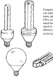
Compact fluorescent lamps (CFL) can replace incandescent lamps in many applications. Although the CFLs cost more initially, they last much longer and cost one fourth as much to operate. They are most effective in areas where the lights are on for long periods.
