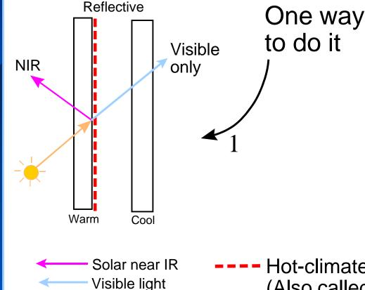
By rejecting nearly half the incident solar radiation with reflection, the SHGC is nearly half as large
