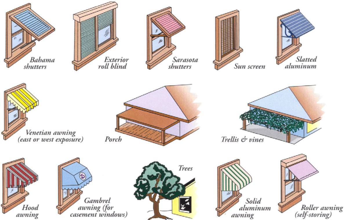
**Figure 4.** The variety of exterior fixed and operable shading devices is large.
