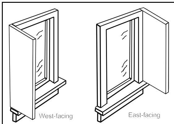
**Figure 3.** Wing walls for shading windows from low sun in summer, without greatly blocking the view.
