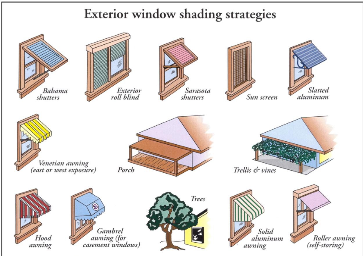
**Figure 4.** The variety of exterior fixed and operable shading devices is large.
